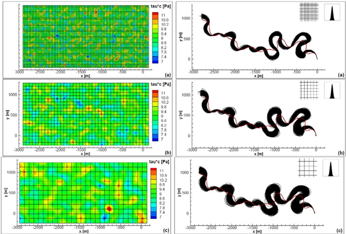
Figure 5 Example realization of floodplain-soil spatial distribution (left) and simulated channel centerline migration (right) for test cases: (a) grid-cell size = 38 m (1 channel width), (b) grid-cell size = 76 m (2 channel widths), and (c) grid-cell size = 114 m (3 channel widths). Flow is from right to left. The initial centerline is colored red and simulated centerlines are colored black.
