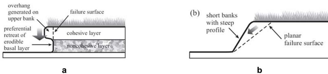
Figure 2 (a) Cantilever failure; (b) planar failure.
