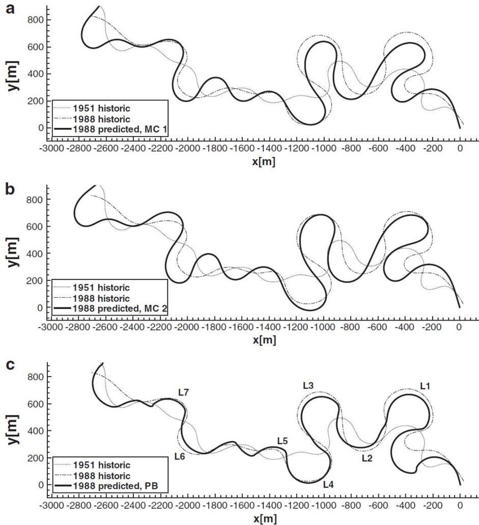
Figure 4 Comparison between historic and simulated 1988 channel centerlines of the Mackinaw River study reach. Flow is from right to left. PB = physically-based method for migration; MC = migration-coefficient method for migration.
