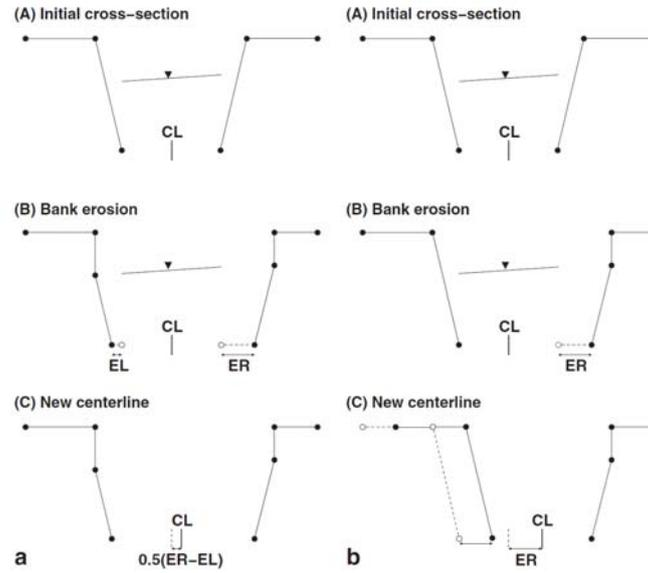
Figure 3 Centerline migration options for the proposed physically-based approach: (a) Option 1 and (b) Option 2. Bank toe displacements ( $EL$  and  $ER$  at left and right bank respectively) determine centerline ( $CL$ ) migration. Alternatively, the intersect points between banks and water surface can be used, instead of the bank toes.
