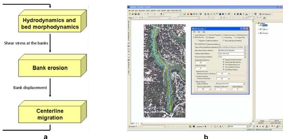
Figure 1 (a) Structure of the RVR Meander platform; (b) interface for ArcGIS-ArcMap.
